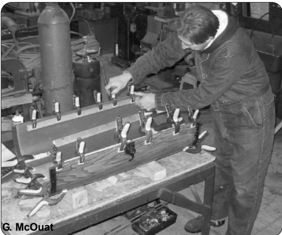
Member Dave Barrett installs a new liner in a K-35 controller cover, which replaces the original "white miracle fibre"
